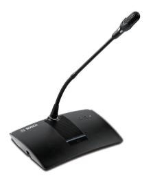
The Delegate Unit with fixed microphone enables participants to speak, register a request-to-speak and listen to the speaker. The microphone stem is flexible. The unit also accommodates two headphone connections, so the speaker can be heard clearly even in situations with excessive background noise. The built-in loudspeaker is muted when the microphone is on to prevent acoustic feedback.
