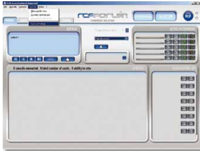
To connect the computer to the control unit, go to the "Options" menu and select "Com port setup" to set the communication port used, entering the number of the port "com" to be used, and then confirm to make the modifications operational. Again from the "Options" menu, select "Connect central unit". The first time the control unit is connected, the following message appears:
