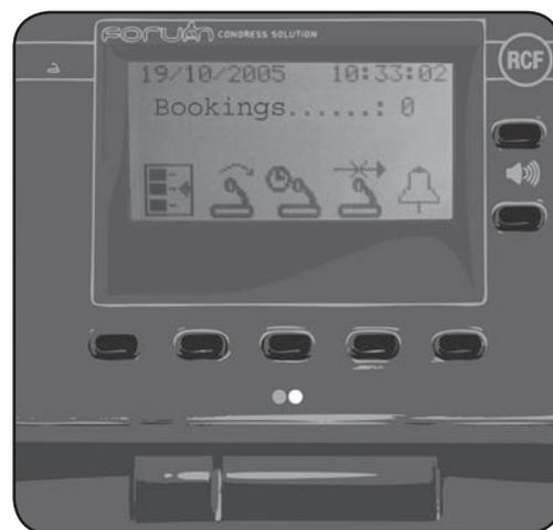
Pressing the key “
