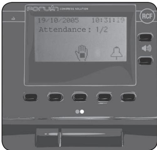
Pressing the key “
