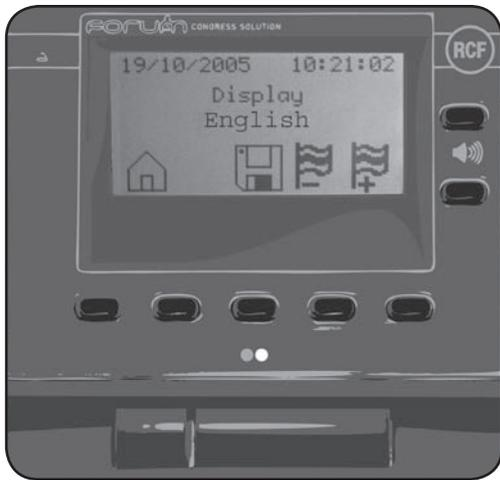
With the smart card, the display language selected using the “set
