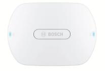
The Wireless Access Point (DCNM-WAP) is the central device of the DICENTIS Wireless Conference System. It links the Wireless Devices (DCNM-WD and DCNM-WDE) by means of secure wireless WPA2 communication. The compact DCNM-WAP with built-in web browser interface is all that is needed to set up, configure and control the DICENTIS Wireless Conference System.
