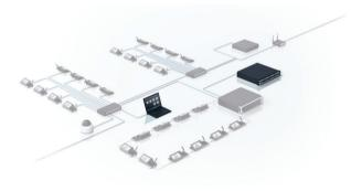
The DICENTIS Camera Control software module makes it possible to interface the DICENTIS Conference System and the DICENTIS Wireless System with Bosch Onvif compliant IP cameras. It selects the activation of fixed or pre-positioned cameras (such as Bosch HD Conference Domes), so that the current active speaker can be displayed during a meeting.
